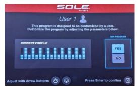
To run the program later, press the USER1 button. A welcome page for SPRINT will be displayed briefly, and then the current profile is displayed. Press Enter or Start to run the program immediately. (NO to RUN PROGRAM only leads to the option to delete the program.)
