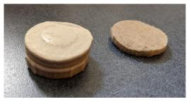
Instead, I tested by trying wooden shims in various positions under the six feet of the machine. I discovered that the problem was completely at the left front of the machine. The feet at the middle and rear of the system are adjustable with a wrench. It
