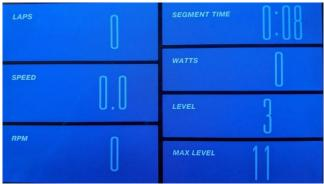
During the workout, pressing the *Display* button, shows some additional data for three seconds. Although the manual is silent on this, a Lap is typically 400 meters (437.4 yards), or possibly 440 yards (quarter mile) in English
