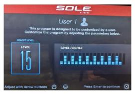
The level for the hard parts is 15, which I just set for the flashing last segment. The level for the easy parts is 5. On the Incline page (not shown), I accepted the default incline of 1 for all segments by repeatedly pressing Enter. Once set up, the program can be run immediately.
