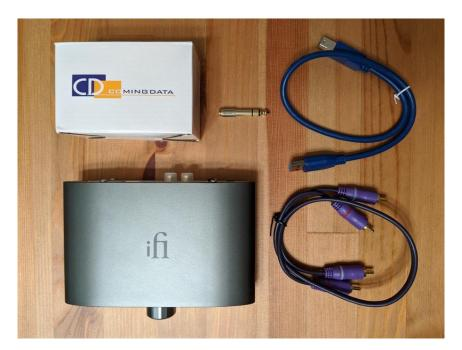
The Zen came with a short USB cable, a short RCA cable, a 6.3 mm to 3.5 mm headphone adapter, and a "manual" on a small card (not shown). The A/C power adapter never left its box, and I did not get to update the firmware.
